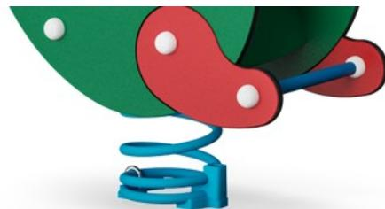
KOMPAN's springs are manufactured from high-quality spring steel. The springs are cleaned by phosphating before being painted with epoxy primer and polyester powder coating. The springs are fixed by unique anti-pinch fittings for maximum safety and longevity.
