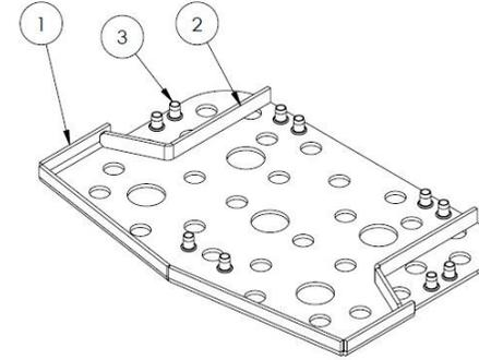
A 5 mm hot-dip galvanized carbon steel plate must be molded inside the SBR to offer optimal stability and optimize the mounting of the step to the frame.
