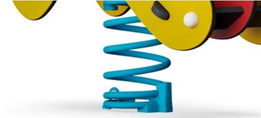
KOMPAN Springs are made of high quality spring steel according to EN10270. The springs are cleaned by phosphating before they are painted with an epoxy primer and a polyester powder coating as top finish. The springs are fixed by unique anti pinch fittings for maximum safety and long lifetime.
