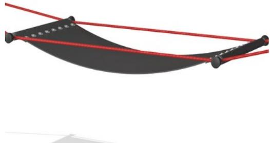
Corocord membranes consist of friction-proof rubberized material of conveyor belt quality with excellent UV resistance. Tested and compliant with REACH requirements for PAH. Embedded is a four-layered armoring made of woven polyester. The armoring and the two surface layers result in a total thickness of 7.5 mm.
