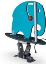
The rocking movement over axis is made by heavy duty scaled ROSTA torsion spring element. The ROSTA element works without any noise and requires low maintenance.
