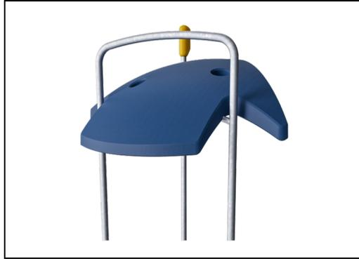
The ELEMENTS roofs are made of recyclable PE made from 33% post consumer recycled materials with a minimum wall thickness of 5 mm to ensure high durability in all climates around the world. The steel pipes are hot dip galvanized inside and outside for maximum durability.
