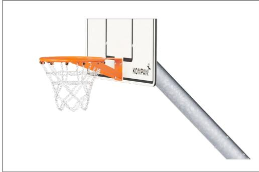
The basketball hoop is made from hot dipped galvanized steel with a powder coated finish. The net is made from Ø4 chain links made from s235 Galvanized steel or stainless-steel chains which meet the requirements in ISO1434-ISO1435 and DIN766. The chains have a circumference of ~Ø30cm at the bottom and ~Ø50cm at the top.
