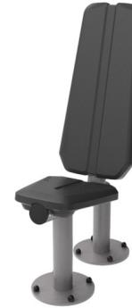
The seat is made of Polyurethane Rubber and has a steel insert plate that is electro-galvanized. The steel plate connects the seat to the frame. This construction makes the seat extremely durable against wear & tear and still very comfortable for a great user experience. The seat is positioned at a height of 46 cm, a comfortable height that makes the transfer from a wheelchair easy.
