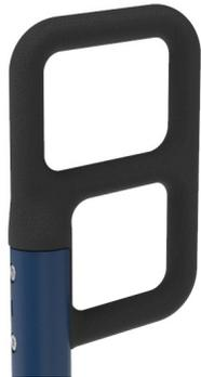
The ergonomically shaped handles have different grip areas for adaptable training, allowing people from 140 – 205 cm tall, to perform the exercise ergonomically correctly and at the same time allowing multiple different exercises. The handles are Aluminum cast and have a diameter of  $\varnothing$  33mm. The Grip Powder coating, used on the support handle, is highly durable against wear and tear, offers isolation, and simultaneously gives users an outstanding grip during their workout.
