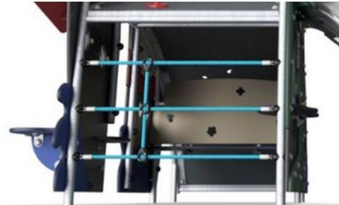
Ropes are made of UV-stabilised PA with inner steel cable reinforcement. The rope is induction treated to create a secure connection between steel and rope, which leads to excellent wear resistance.
