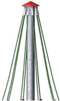
In the centre of the Spire net is the mast, made of high-quality seamless steel. The structure of the mast as an oscillating support which is statically favourable and equalises the oscillations in the Spire Net. The masts are hot-dipped galvanised as standard.
