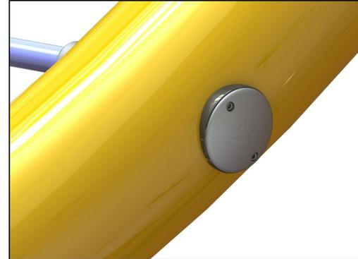
The rope is fixed to the large steel pipe by a unique KOMPAN designed tightening solution. It consists of inner and outer nylon (PA6) bushings that guides the rope to an outside threaded stainless steel part that tightens the rope.
