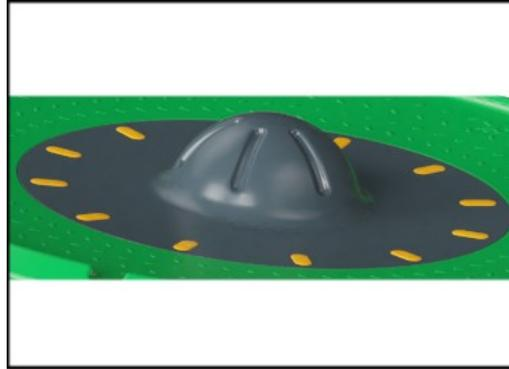
The center part of the bowl is made of recyclable LDPE and fixed to the outer ring by 12 attachment points sealed with yellow PA nylon caps.
