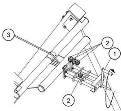
The steel cable 3 is tensioned by a special designed device. By turning the handle 1 the steel cable can be tensioned according to instruction in a safe way. After tensioning the cable is locked by three clamps 2. The tensioning device can also be used for adjustment during annual inspections.
